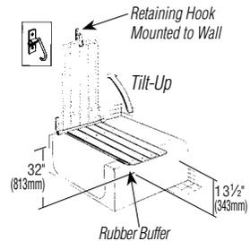
Retaining Hook Mounted to Wall
