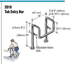
This bar provides a convenient grip for balance at tub entrance. The time-tested design combines floor mounting with a brace that adjusts against the tub for a snug fit. Note: Dimensions are for 16" (406mm) tub height. If different, please give tub height from floor.
