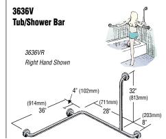
The 2040V and 3636V are excellent multi-purpose bars that provide a vertical arm and two horizontal supports for added stability. When entering tub, if the bather's right hand grips the vertical, specify right hand. If reverse, specify left.
