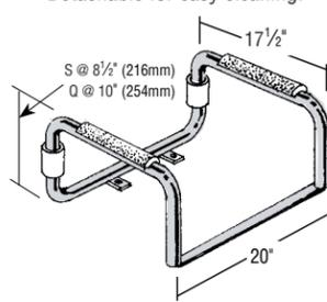
Extra-wide legs for easy access by wheelchair users. The 1822-F mounts to the floor and the 1818-FM-3 tilts up for easy cleaning. Both bars fit toilet bowl height of 15" - 15 1/2" (381-394mm), but can be modified to fit your requirements.
