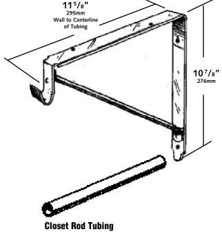
**CQ-6** - 6' (1829mm) **CQ-12** - 12' (3658mm) TSM will cut to fit as specified.
