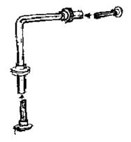
Use grab bar as a template to pinpoint mounting hole placement. Bolt bar to wall and floor.
