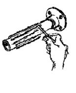
Slide cover flange over each end of bar. Insert internal steel liners at each end of bar while adhesive is still wet and fresh.
