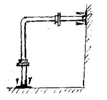
Apply a dab of adhesive 1/2" away from ends of bar, then slide cover flange over base plate. Make sure the cover flange touches the wall or floor. Allow four (4) hours for the adhesive to dry.
