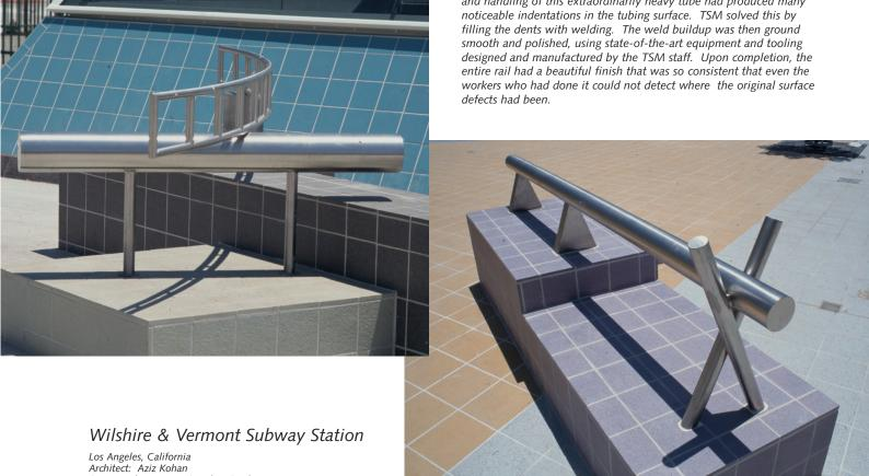
Satin Finish Type 304 Stainless Steel Bench at Left : Tubing 8" O.D. x .120" (203x3mm), Posts 2<sup>1</sup>/<sub>2</sub>" x .120" (64x3mm) Curved Ladder 1" O.D. x .120" (25x3mm) Bench at Right: Tubing 6" O.D. x .120" (152x3mm) and 3" O.D. x .120" (76x3mm) Triangle Posts 1/8" Plate (3mm) Left, Model #GRD-822 Right, Model #GRD-827
